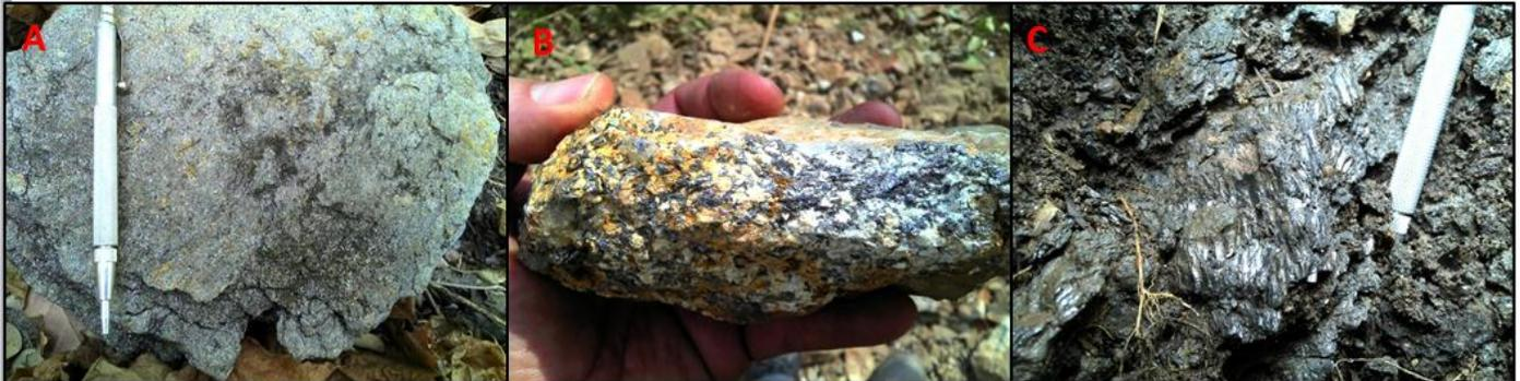
**Figure 2. Three main varieties of graphite mineralisation at Nachingwea. A - graphite-quartzite, B - graphite-gneiss and C - semi massive graphite schist**
